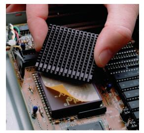
Bergquist CPU Pad is a thermally conductive, electrically insulating, double coated tape. The tape consists of a high performance acrylic, pressure sensitive adhesive, on both sides of a film. This product can be used in applications that currently require clips. CPU Pad is typically used to mount a heat sink on top of a central processing unit on the circuit board.
